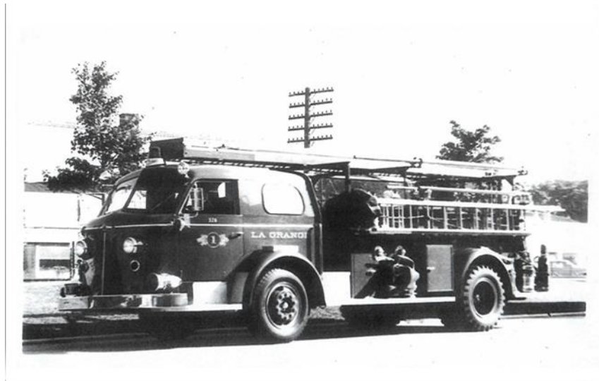
ENGINE CO. 326 IS A 1951 AMERICAN LA FRANCE PUMPER WITH A LEFT SIDE MOUNTED PUMP PANEL. THE LADDER RACK ON TOP IS NOT ORIGINAL, IT WAS ADDED LATER AND CARRIED A 35' LADDER WITH TORMENTORS POLES. THIS VEHICLE SERVED THE RESIDENTS OF LA GRANGE UNTIL 1981.
